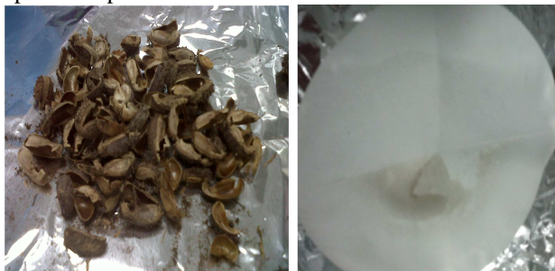
Fig. 1. Photos of CS (a) before treatment and (b) after the treatment (cellulose)
